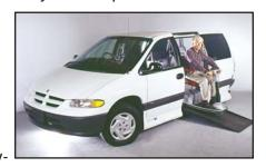
ered floor that allows the vehicle to be parked in a garage. Although it varies, the lowered floor van allows approximately 2" less interior headroom than the full size van. Mini vans are usually equipped with an automatic ramp that is an integral part of the vehicle. As the ramp automatically unfolds, the kneeler allows the rear of the vehicle to lower resulting in a very gradual incline to the entry ramp.
